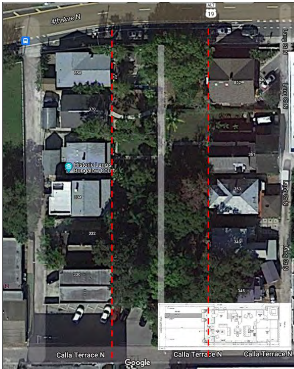
Figure 1: Setback line of existing contributing resources with proposed site plan (not to scale). Aerial image via Google Earth.
